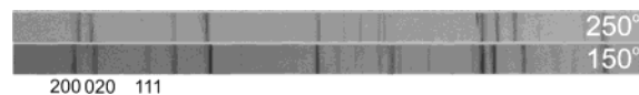
Figure 1. High-temperature XRD patterns of \text{Na}_4\text{VO}(\text{PO}_4)_2 taken in a Guinier-Lenne camera at 150 and 250 \text{ }^\circ\text{C} .
